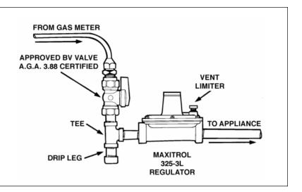
At supply pressures above 2-psi, the new standard requires the use of an over-pressure protection device (OPD) for use with the regulator. (See below.)
