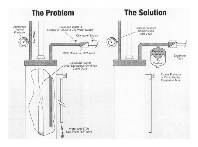
The Problem: In the "Good Old Days", before the advent of cross-connection control, expanded water which exceeded the capacity of the water heater flowed back to the City main where it was easily dissipated. But today, with the backflow preventers, water meters with check valves, and/or pressure reducing valves without bypass being installed, expanded water from a water heater cannot return to the City supply. It is now a closed system, and the expanded water has no place to go.
