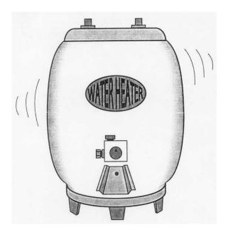
When dual-check valves and check valves are installed in water meters, they seal off the household plumbing system from the potable contaminated household water into the public supply. Because they do their job so well, these backflow devices can contribute to thermal expansion, which can cause serious problems.
